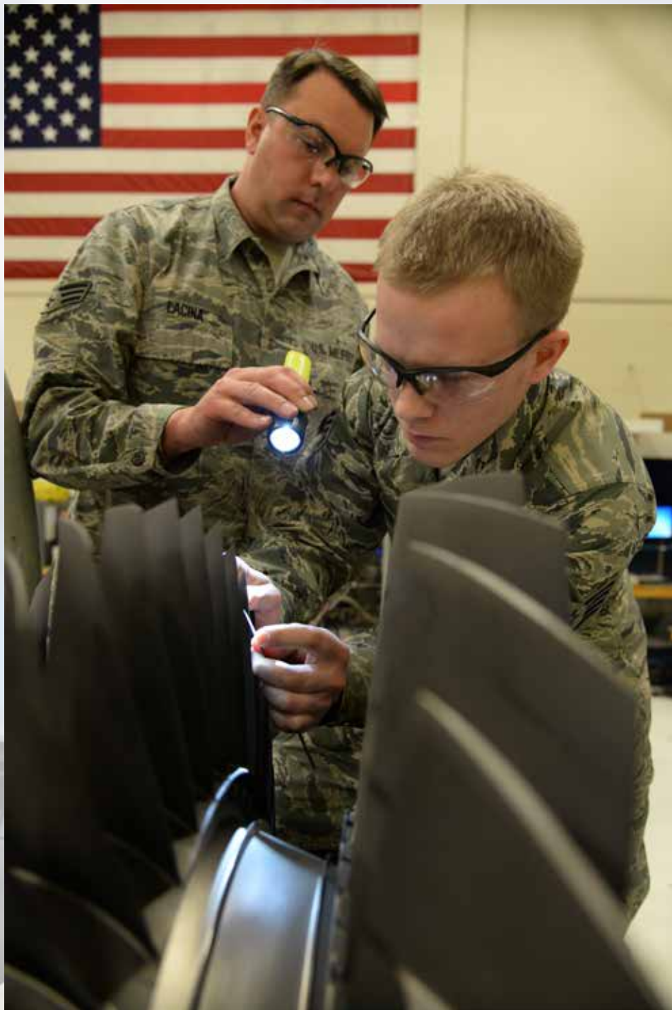
Senior Airman William Lacine and Staff Sgt. Matthew McEwen, 148th Fighter Wing Engine Shop blend second stage fan blades on an F-16 engine, March 7, 2015, Duluth, Minn. These routine inspections are in place to catch problems when they are small and fix them before they blossom into much bigger problems. (U.S. Air National Guard photo by Master Sgt. Ralph J. Kapustka)
